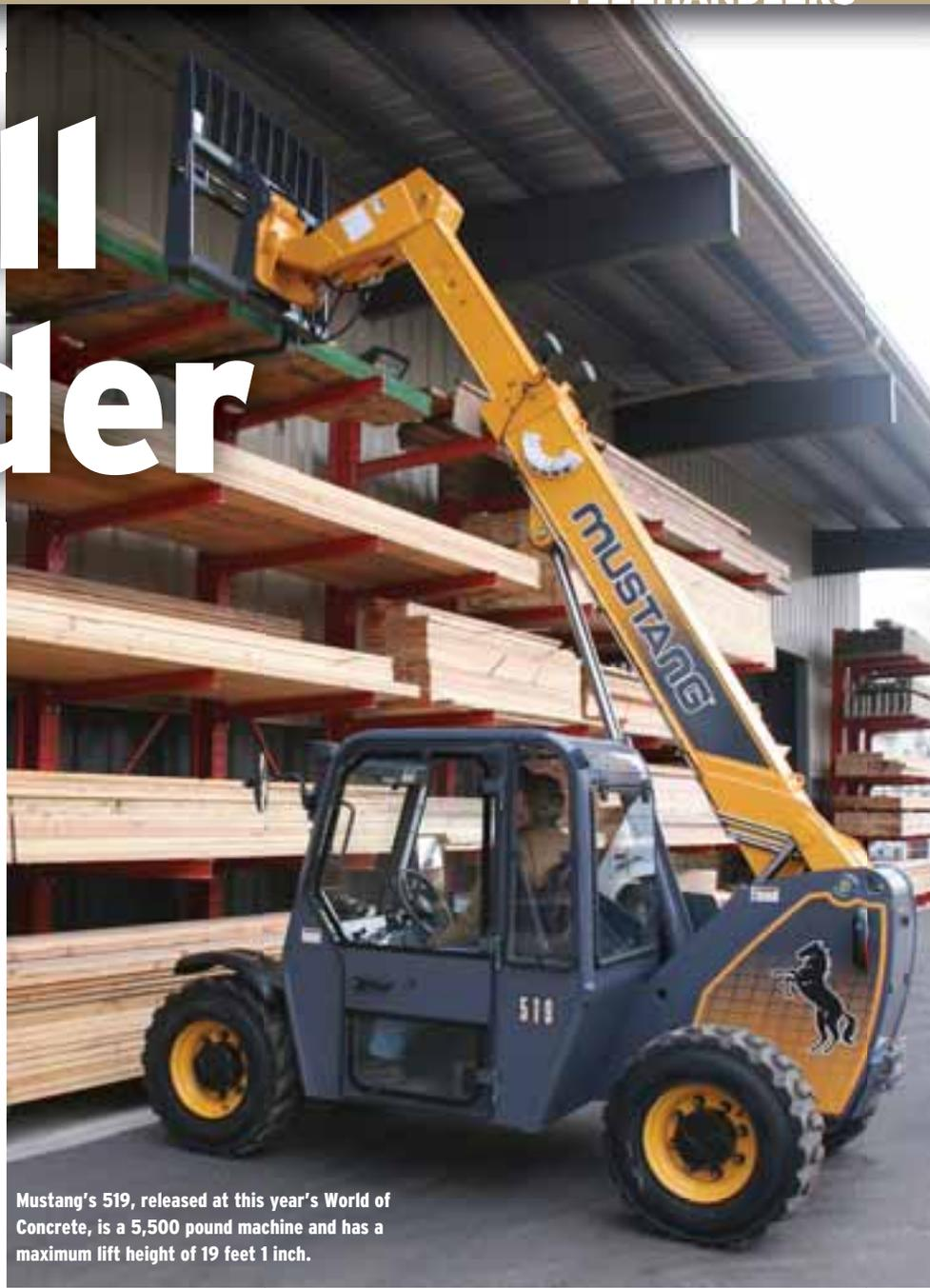
Mustang's 519, released at this year's World of Concrete, is a 5,500 pound machine and has a maximum lift height of 19 feet 1 inch.
