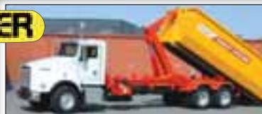
Palift is Palfinger's line of heavy duty multi purpose hook lifts. Palift offers capacities from 9,000# to 68,000# and dump angles to 57 degrees.
